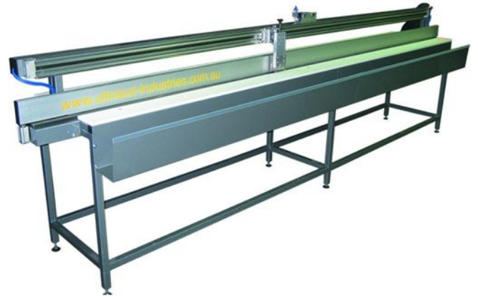
PRCR01- Low Cost Combination machine PRESSURE CUTTING & CREASING
